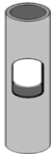
Fig. 1: Schematic diagram of slotted tube specimen used for uniaxial loading total-life fatigue studies; not to scale.
